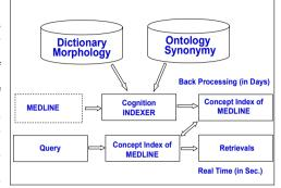
The CSIR Indexer uses its NLP component to build a cognitive model of the text in which all of the concepts (word meanings) of a document are indexed as well as word strings. The NLP component relies on its dictionary, semantic map, and morphological and syntactic tags. At search time, CSIR interprets the query meaning, and searches for this meaning in its concept index rather using statistical word pattern matching. Therefore, the results are more complete and relevant.
